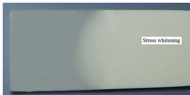
Figure 5. Stress whitening resulted from the cavitation and orientation. [Color figure can be viewed in the online issue, which is available at wileyonlinelibrary.com .]
